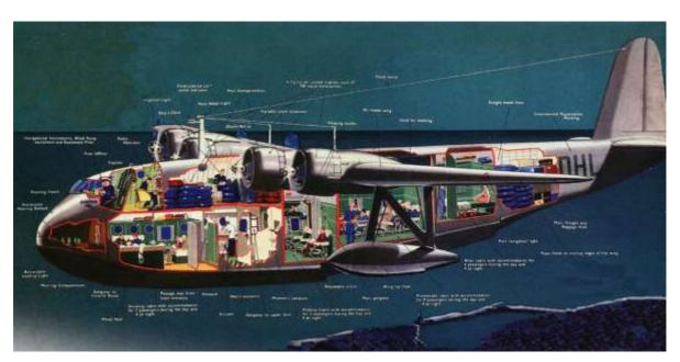
Cutaway view of an S.23 Empire boat. Clearly shown is the double deck layout with the Flight Clerk (later redesignated as Purser), located at the rear of the flight deck. Due to larger than anticipated volumes of EAMS mail and freight being uplifted, his station was repositioned in the forward passenger cabin.
