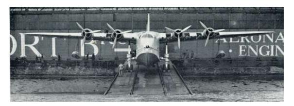
Canopus, the first of the "C" Class flying boats on the slipway prior to her first flight standing on her beaching gear. Just visible are five open maintenance platforms built into the wing leading edges (four starboard and four port).
